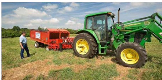
ARS soil scientist Dan Pote observes as ARS technician Stephen Haller operates their invention, the Poultry Litter Subsurfer—the first commercially viable machine for applying dry poultry litter below ground.
