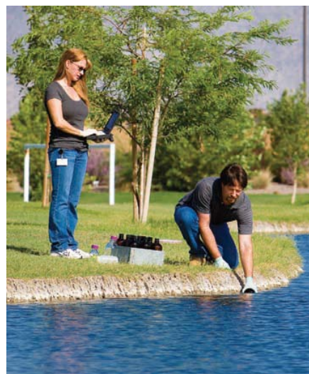
Technicians Allan Knopf and Sharette Evans collect water samples from a pond that supplies irrigation water to Pacana Park in Maricopa, Arizona. In the laboratory, the pond-water samples are tested for presence of humanspecific Bacteroides molecular markers.
