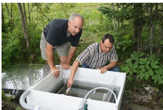
ARS agricultural engineer Kevin King (right) and soil scientist Jim Balogh, of Spectrum Research, Inc., inspect a filter cartridge system being evaluated at a golf course tile drainage site. The cartridge system was donated by cooperating industry Kristar Enterprises, Inc.
