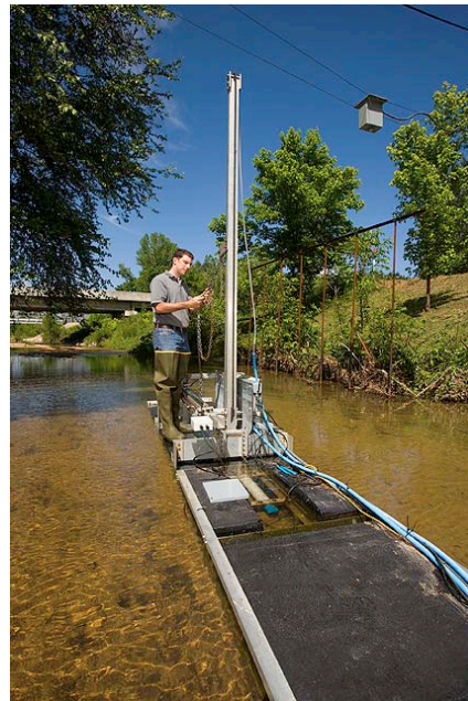
Hydraulic engineer Daniel Wren makes adjustments to the floating instrument platform used in Goodwin Creek Experimental Watershed near Batesville, Mississippi. The platform is used for data collection and development of acoustic technology for field measurement of sediment transport.
