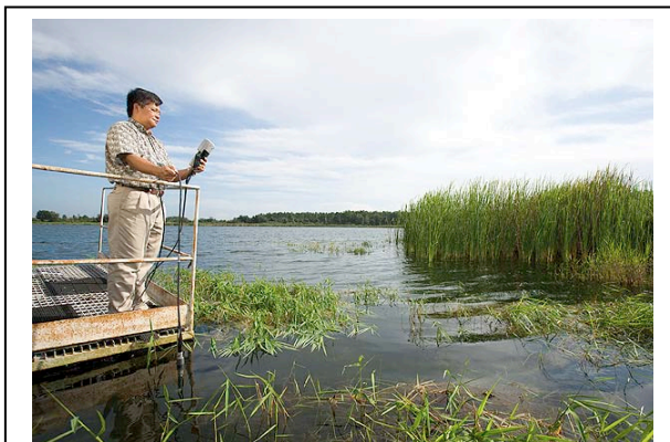
Soil scientist Gilbert Sigua uses a probe to measure levels of salinity, dissolved oxygen, conductivity, and temperature in Spring Lake, in Brooksville, Florida. The lake is located near forage-based cow-calf operations.
