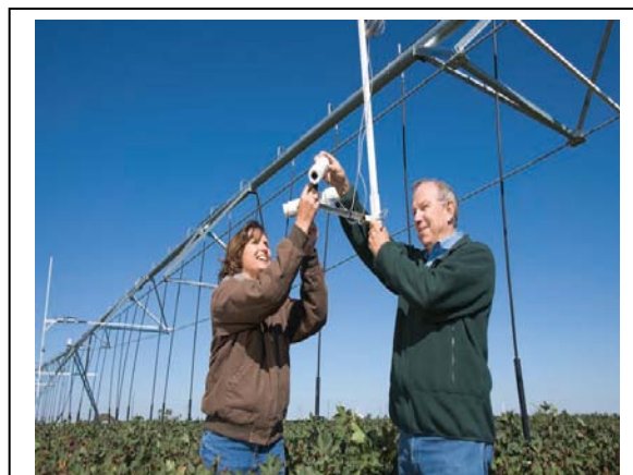
Agricultural engineers Susan O'Shaughnessy and Nolan Clark adjust the field of view for wireless infrared thermometers mounted on a center pivot irrigation system. The wireless sensors are used to measure crop canopy temperature for indications of water stress.
