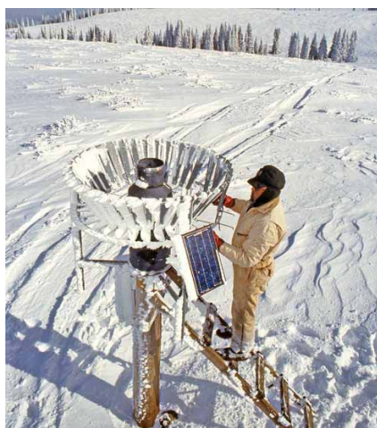
A technician examines the snowfall collected in a precipitation gauge on the solar-powered telemetry system at the Reynolds Creek Watershed.
