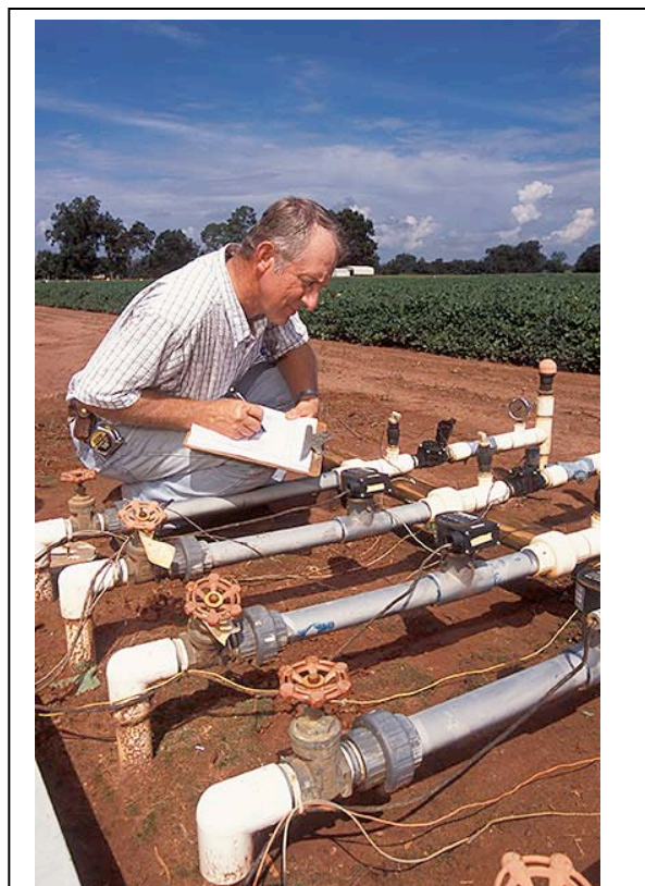
Technician Ernest Yoder checks waterflow instrumentation on a subsurface drip irrigation system used for peanuts, cotton, and corn crops.
