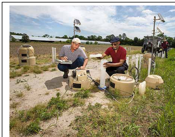
Soil scientist Ray Bryant (left) and UMES researcher Arthur Allen collect samples of groundwater before and after it is filtered through an underground “curtain” of gypsum. Dissolved phosphorus in groundwater is reduced after flowing through this setup.
