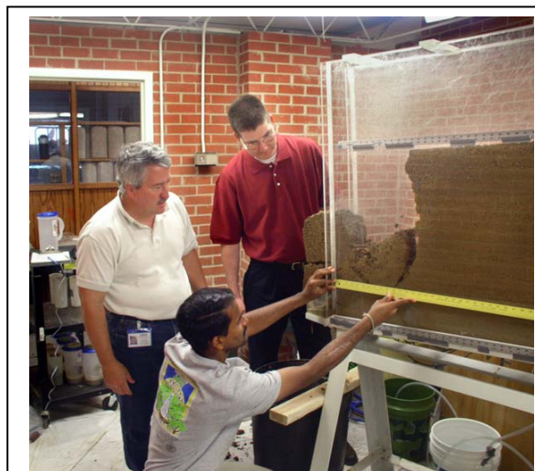
ARS hydrologist Glenn Wilson (left), graduate student Raja Periketi (center), and Oklahoma State University scientist Garey Fox use a simulated streambank to conduct laboratory experiments of seepage erosion on streambank failure. Periketi is measuring the lateral extent of a mass failure caused by seepage erosion.
