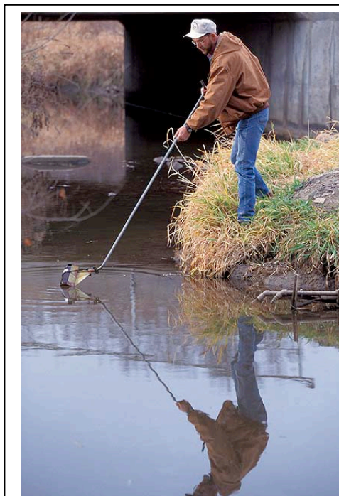
Many CEAP watersheds use the SWAT computer model to predict effects of farm practices on water quality. Here, technician Jeff Nichols collects a sample from a watershed in Ames, Iowa, as part of earlier work to refine the model.
